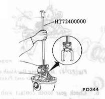
Fig. PD-44 Removing Differential Assembly Case
