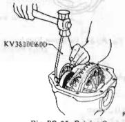
Fig. PD-65 Driving Spacer Into
