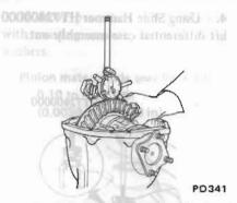
Fig. PD-41 Measuring Backlash of Ring Gear and Pinion
